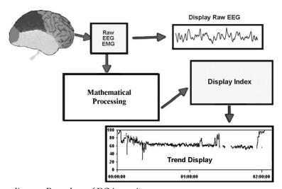
Fig. 1. Flow diagram Procedure of DOA monitors
