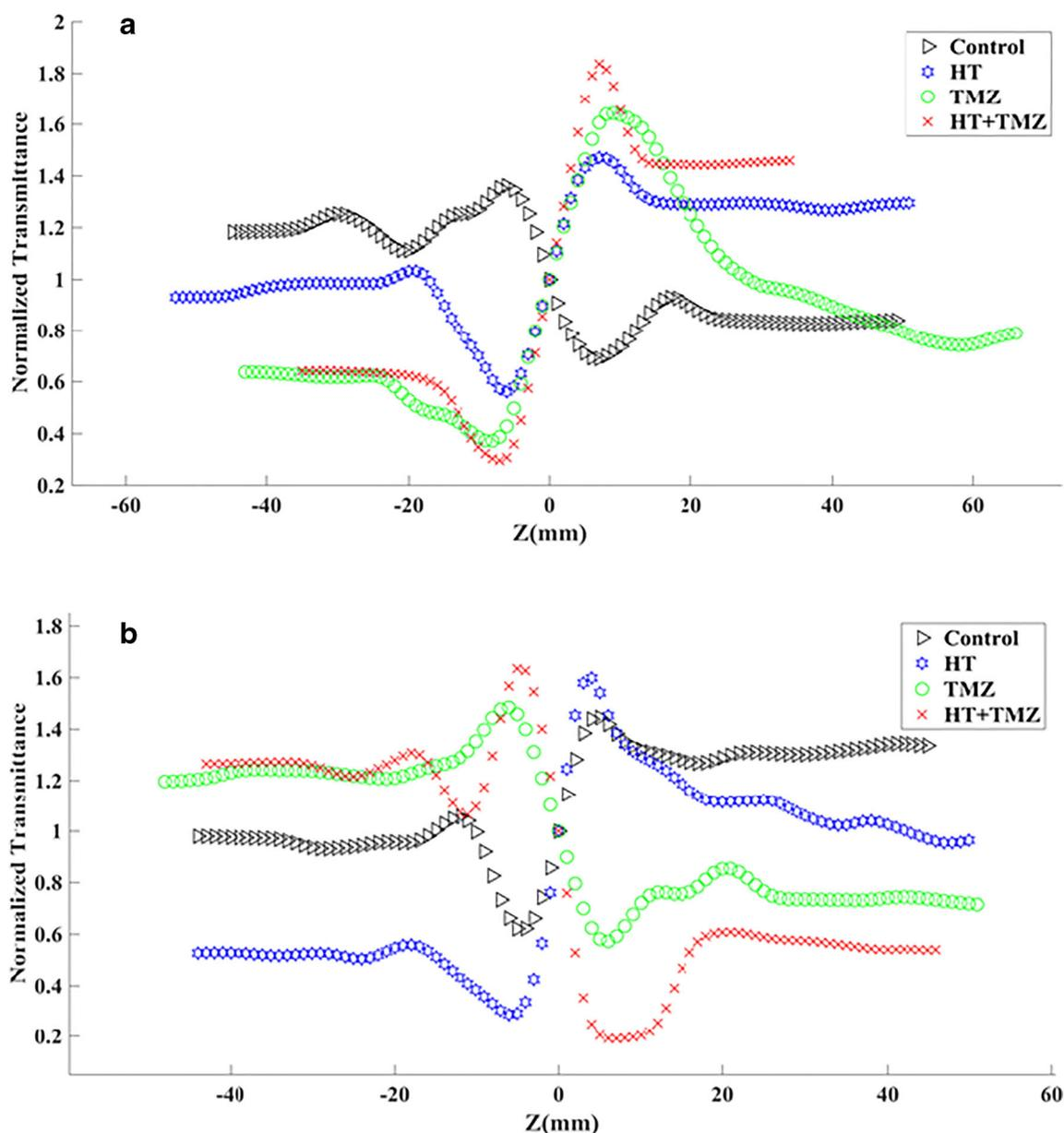
**Fig. 4** Closed aperture Z-scan normalized data for **a** C6 glioblastoma and **b** OLN-93 glioma cell lines for different treatments. Normalized transmittance represents transmittance power changes through the aperture according to the sample position and was measured by detector
