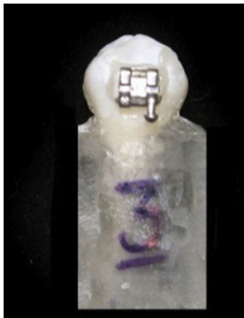
Fig 2. Mounted tooth in acrylic block after bonding.
