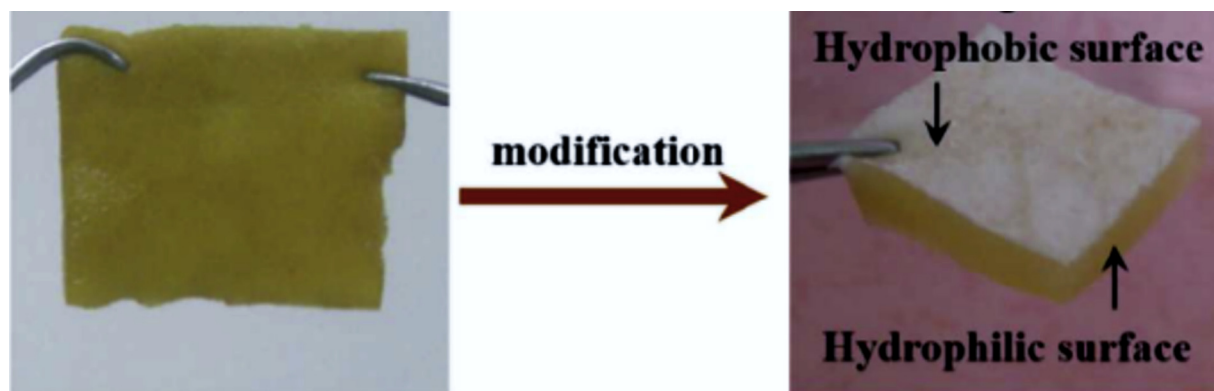
Fig. 7. Photographs of asymmetric wetting modification with hydrophobic and hydrophilic surface (Reprint license number: Adapted with permission from Ref. (Liu et al., 2009) Copyright 2016 American Chemical Society).
